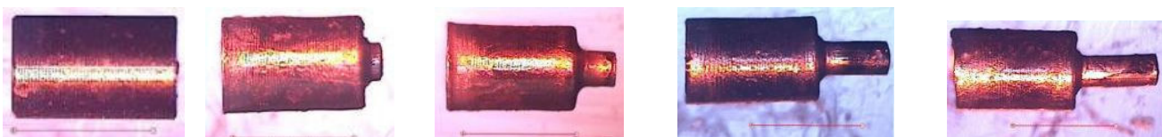
Extrusion of components from 0 to 0.90 mm. The line below each component represents 1mm.
